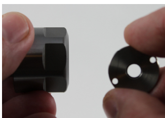
Thread Coolant Cap into ER nut, snug with wrench after the collet has been assembled.
