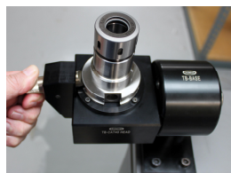
Insert Holder into Assembly
