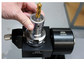
Assemble cutting tool, snug by hand to hold the cutter in place
