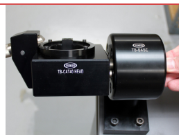
Rotate the knob to the desired location, the head will lock in 90 degree increments
