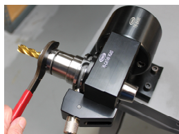
Rotate the Head to the 270° position to tighten the locking nut
