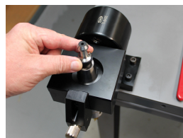
Rotate to the 180° position to install and tighten retention knob
